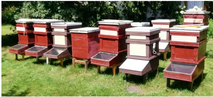
Figure 2. Experimental apiary consisting of prototypes of the Solar Hive and the latest models. The objective is to study temperature regimes inside the hives under various weather conditions, as well as the response of bees to temperature effects of varying levels.
